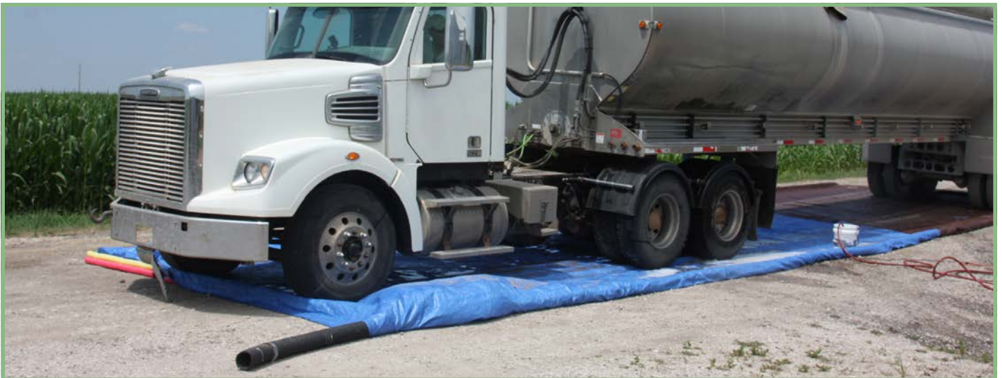
Use stakes to secure the tarp to the ground through the grommets if surface allows
